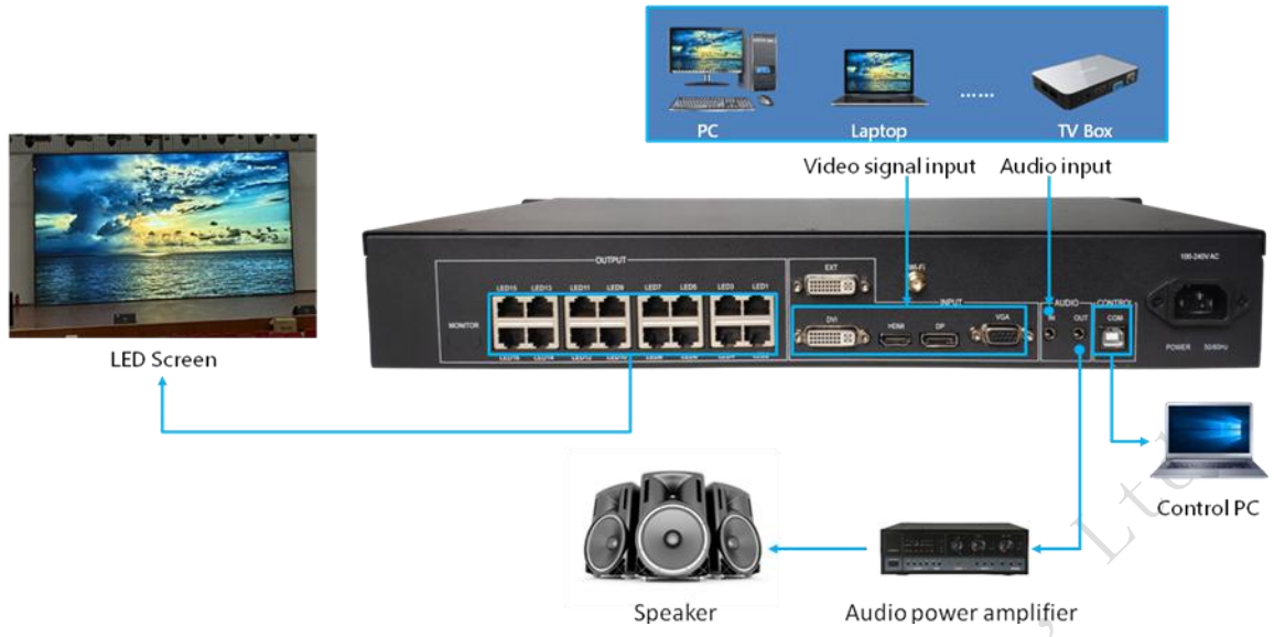
Connection diagram
