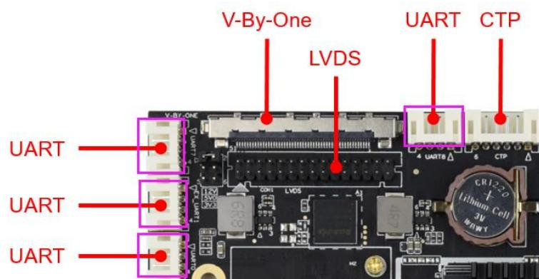
The board have two sets of ordinary UART serial ports, which can support the UART serial port devices on the market.
