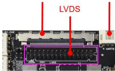
General LVDS interface definition, support single / dual, 6/8 / 10-bit 1080P LVDS screen. The screen voltage can be selected through a jumper cap, and it can be selected to support 3.3V / 5V / 12V screen power supply.
