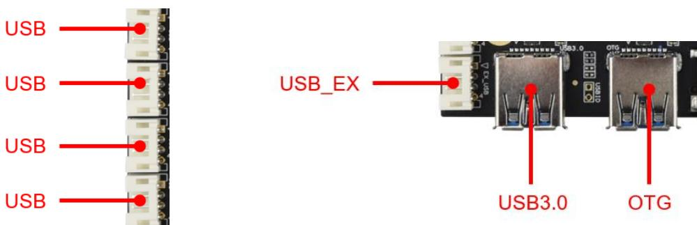
The board has 2 USB standard interfaces and 4 USB pins, one of which is shared with the 4G module.
