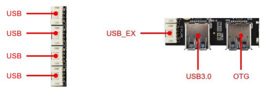
The board has 2 USB standard interfaces and 4 USB pins, one of which is shared with the 4G module.
