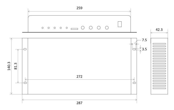
Tolerance: ±0.3 Unit: mm
